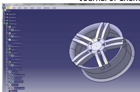
Figure.3. CATIA Model of 5 Spoke Rim
